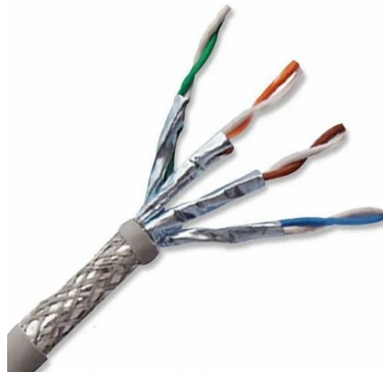
Figure 5 – multiconductor STP example with 4 STPs, wrapped with conductive mylar, outer shield, reinforcing metal braid, and insulating jacket
